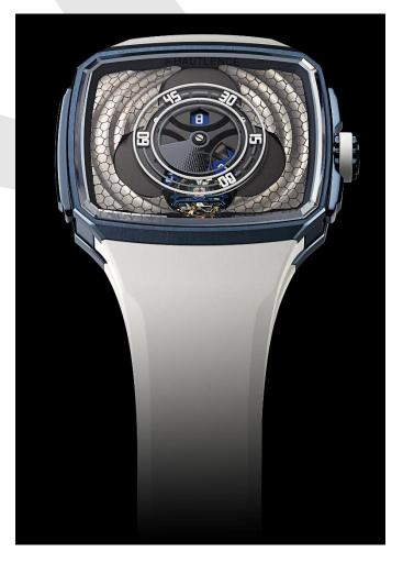
superconductor is cut across the grain at a specific angle. The material is then soaked in an acid bath, which attacks the copper but leaves the niobium intact, revealing a stunning, contrasting, tight honeycomb network. The result is a unique and almost organic lattice of raw metal.
